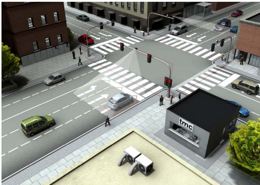
Verification and viewing of the vehicle presence detection zones can be done from the TMC.
